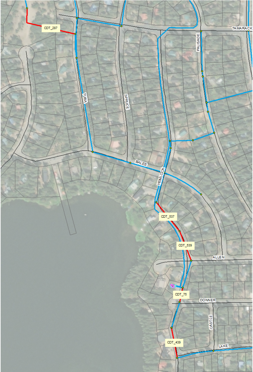
Figure 14: Existing Collection System – Highest d/D Values
